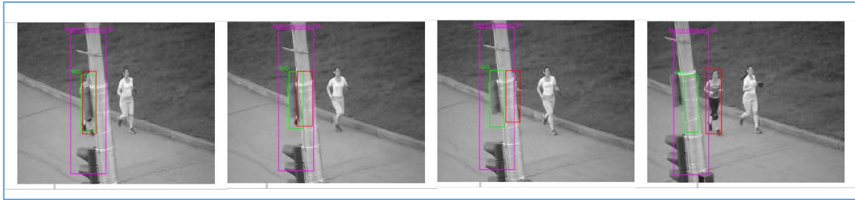
FIGURE 25 – JOGGING: USING HOG ONLY FOR OBJECT TRACKING (FRAMES 68, 71, 73, 86)
