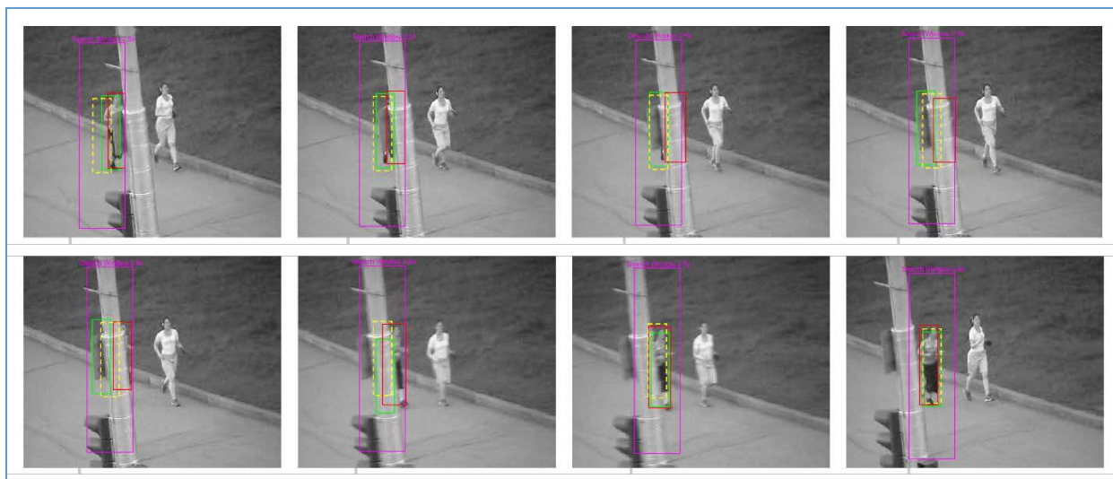
FIGURE 27 - JOGGING SEQUENCE USING HOG TO INFORM AN ADAPTIVE KALMAN FILTER.
