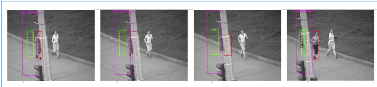
FIGURE 26 - JOGGING: HOG+NON-ADAPTIVE KALMAN FILTER TRACKING (FRAMES 68, 71, 73, 86).
